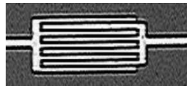
Fig. 2. Top-view microscope image of a single comb-shaped sensor structure (aluminum) in the top metal layer of the IC.
